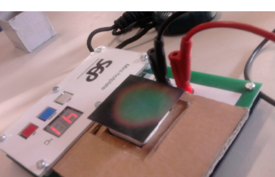
Heat conduction: evaluating aerogels as insulators with LCD sheets
